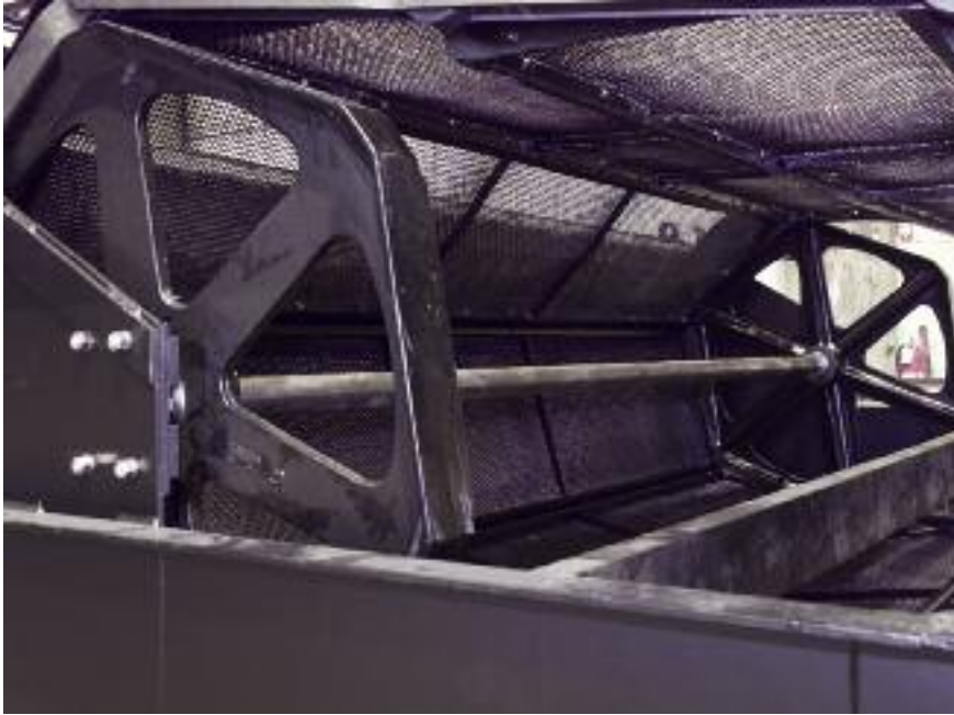
Rebuilt screens are fully disassembled, blasted to bare metal, and reassembled with new wear components, ready for extended service at your intake.
